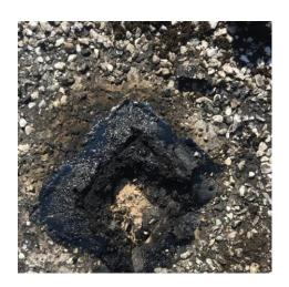
Core sample of Asphalt roof
